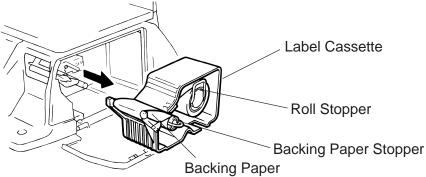
**NOTE:** When removing the backing paper, loosen the paper by turning the paper winding shaft counterclockwise.
